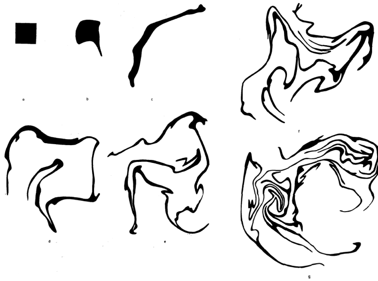
Figure 1–1: Deformation of a fluid element as observed by Welander ( Welander , 1955) in a film of buthanol over water. The size of the tank is 50 \times 30 \times 30 cm. The flow is lamellar and the tank is rotating to keep the motion two dimensional.
